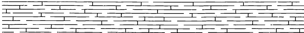
Fig. 9.5 Cross-linking long molecular chains by covalent bonds increases rigidity of a plastic.
